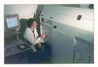
Plate 11. Inductively-coupled plasma/mass spectrometer
