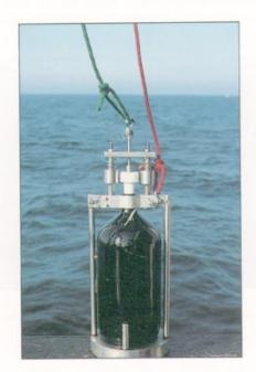
Plate 8. Surface water sampler (2.5 l)
