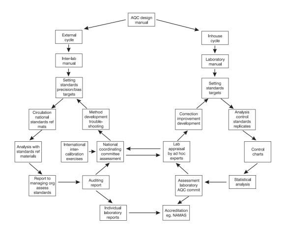
Figure 2. NMAQC Scheme operation (idealised approach)
