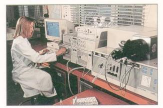
Plate 12. Coupled high-performance liquid chromatograph/mass spectrometer
